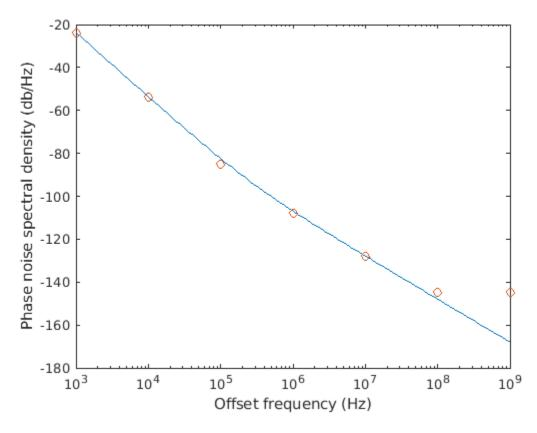
It appears that there is a measurement noise floor at -140 dBc/Hz for the specification dataset, and the phase noise for the device under test is probably below that noise floor for offset frequencies above 100 MHz. In this case, a set of parameter values that fit best to the data at lower frequency offsets is likely to produce a more accurate model.
