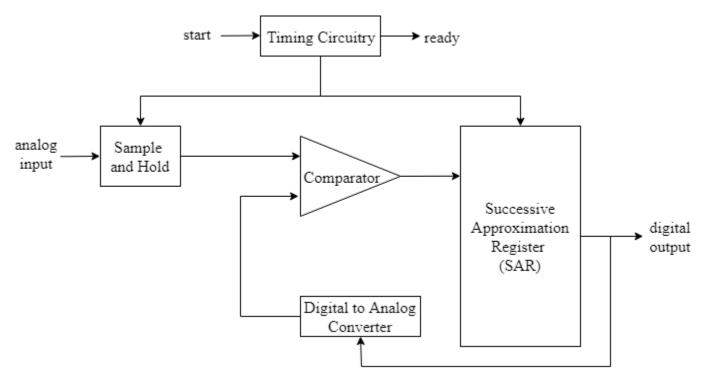
When the ADC receives the **start** command, SHA is placed in hold mode. The most significant bit (MSB) of the SAR is set to logic 1, and all other bits are set to logic 0.
